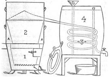
The portable furnace (1) is most excellent for boilers of from 5 to 10 gallons, and may be used as a heating or cooking stove for families, as well as for the purposes of distillation. Coal can be filled in without moving the boiler, it having a good draught of air, and being laid out with firebricks, with a fall-grate for extinguishing the coal after using. The above can be obtained, ready-made, of J. Murphy, at No. 256 Water street, complete for \$5.
